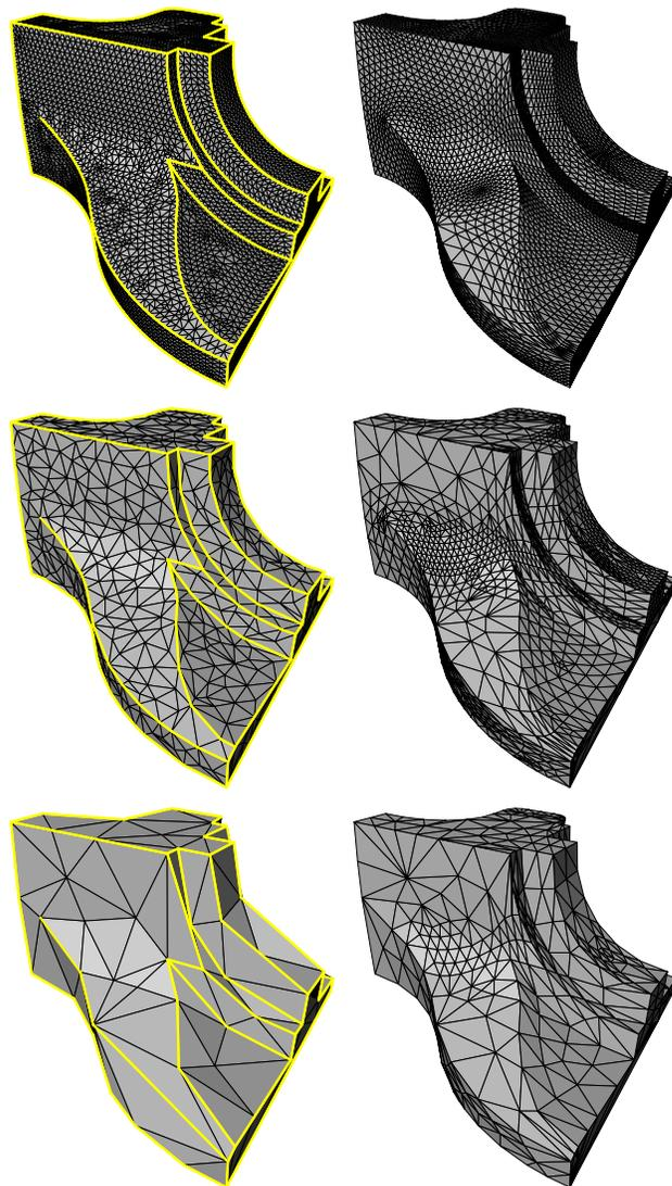
Figure 13: Left (top to bottom): three levels in the DK pyramid, finest ( $L = 15$ ) with 12946, intermediate ( $l = 8$ ) with 1530, and coarsest ( $l = 0$ ) with 168 triangles. Feature edges, dart and corner vertices survive on the base domain. Right (bottom to top): adaptive mesh with  $\epsilon = 5\%$  and 1120 triangles (bottom),  $\epsilon = 1\%$  and 3430 triangles (middle), and uniform level 3 (top). (Original dataset courtesy University of Washington.)
