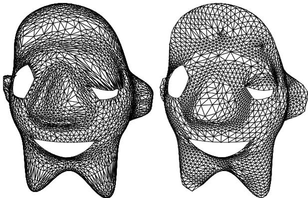
Figure 12: Example remesh of a surface with boundaries.
