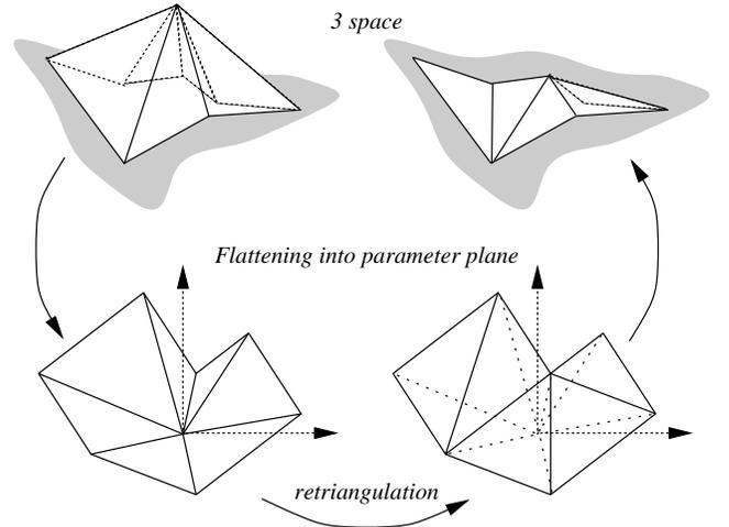
Figure 5: In order to remove a vertex  $p_i$ , its star  $(i)$  is mapped from 3-space to a plane using the map  $z^a$ . In the plane the central vertex is removed and the resulting hole retriangulated (bottom right).
