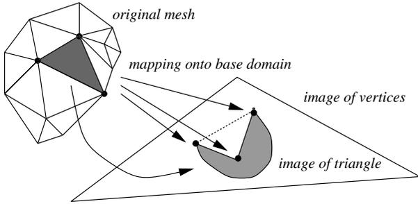
Figure 8: Although the mapping  $\Pi$  from the original mesh to a base domain triangle is a bijection, triangles do not in general get mapped to triangles. Three vertices of the original mesh get mapped to a concave configuration on the base domain, causing the piecewise linear approximation of the map to flip the triangle.
