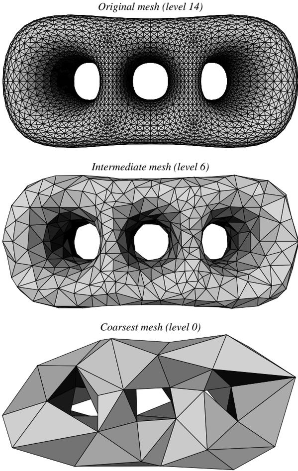
Figure 4: Example of a modified DK mesh hierarchy. At the top the finest (original) mesh  $\phi(|\mathcal{X}^L|)$  followed by an intermediate mesh, and the coarsest (base) mesh  $\phi(|\mathcal{X}^0|)$  at the bottom (original dataset courtesy University of Washington).
